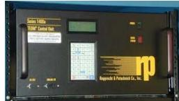
Avtomatski merilnik  $\text{PM}_{10}$
